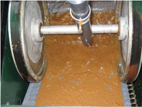
Image 5. Dewatering of coagulated iron in the Self Indexing Filter.
