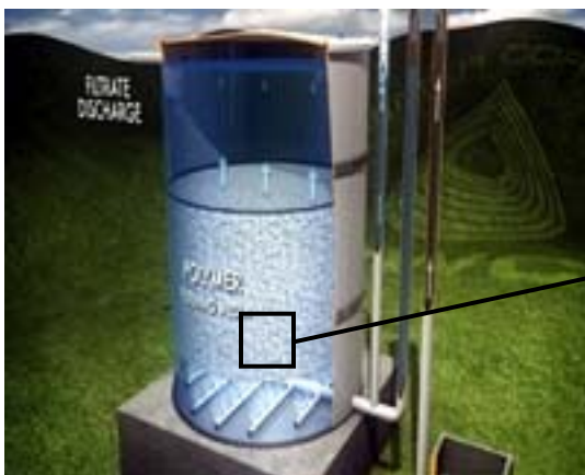
Image 1. Permanent Media Filtration within DEFERUM™ hydro-automatic filter.
