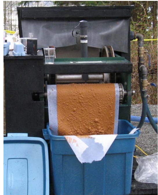
Coagulated Iron being removed from Self-indexing Filter
