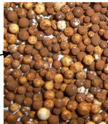
Image 4. Close-up of media following absorption of Iron
