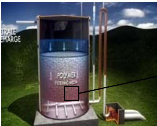
Image 3. Automatic Backwash Stage within DEFERUM™ hydro-automatic filter.
